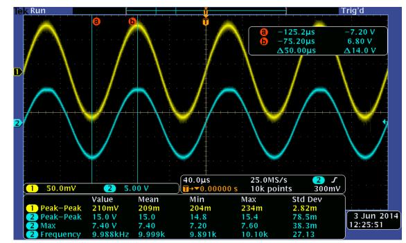
4. Clipping on one peak at Vin = 209 mVpp, Vout = 15.0 Vpp. Vout is clipping between 6.80 V (cursor) and 7.40 V (Max).
