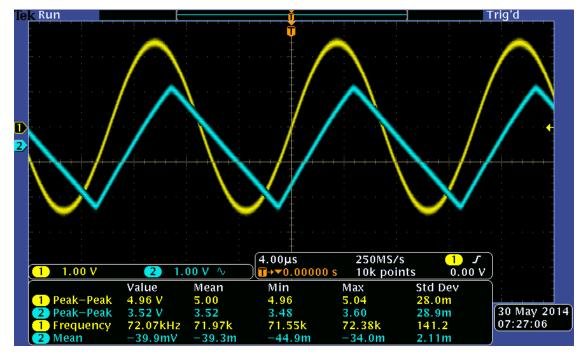
Shown here (not required), we begin to hit the slew rate at about 31 KHz for Vin = 5.0 Vpp.
