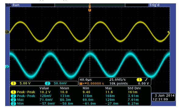
6. Set Vin- = Vin+ = 10 Vpp, 1.0 KHz sine wave, 0 V DC offset. Shown here, Av(common mode) = 131 mVpp / 10.0 Vpp = .013.
