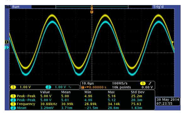
Increase Vin until clipping begins. Shown here, it's clipping negative at Vin = 13.0 Vpp, Vout = 12.0 Vpp. (I should have let the mean settle, so I'm using the current value, which better matches the trace.) You may not be able to get your circuit to clip if your function generator doesn't go high enough.
