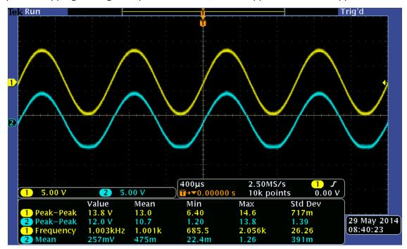
4. Continue increasing the amplitude of Vin until Vout begins clipping on the other peak. Clipping on both peaks occurs at Vin = 16.8 Vpp, Vout = 13.9 Vpp.
