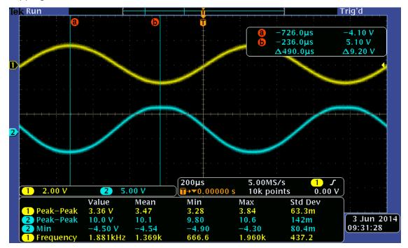
Clipping on negative peaks happens at Vin = 3.71 Vpp and Vout = 10.3 Vpp. Positive peaks are clipped between 5.10 V (cursors) and 10.3 – 4.69 = 5.61 V (P-P + Min). Negative peaks are clipped at between -4.30 V (cursors) and -4.69 V (Min).
