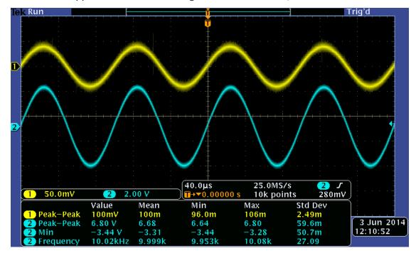
2. Ground Vin– and set Vin+ = 100 mVpp, 1 KHz sine wave, 0 V DC offset. (This shows Vin = 100 mVpp *at 10 KHz*; I've changed the instructions.) Av = 66.8 = 36.5 dB.
