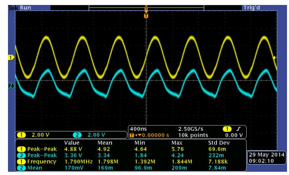
2. Find the 3 dB point. For my circuit, this would be where Av = .7071 \* .99 = .70. Shown here, Av = 3.34 / 4.92 = .68 at 1.8 MHz. But note the distortion.
