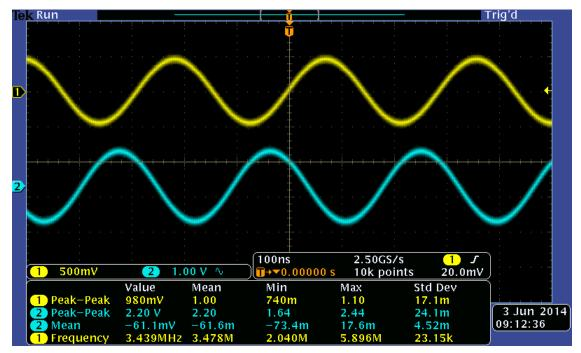
5. Onset of clipping on positive peaks happens at Vin = 3.47 Vpp and Vout = 10.1 Vpp. Clipping is at Vout between 5.10 V (cursors) and 10.1 - 4.54 = 5.56 V (P-P + Min).
